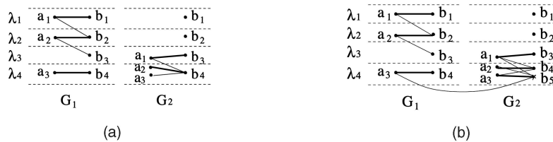
Fig. 4. (a) Fig. 3 is decomposed into two subgraphs when only considering the output vertices. (b) Assigning a buffer vertex on \lambda_4 to G_2 .
