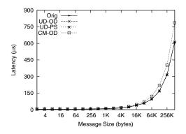
Fig. 7. Latency of Different Connection Management Algorithms
