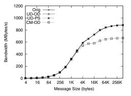
Fig. 8. Bandwidth of Different Connection Management Algorithms
