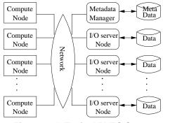
Figure 9. A Typical PVFS Setup
