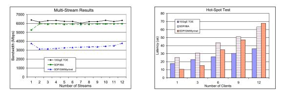
Figure 5. Multi-Connection Micro-Benchmarks: (a) Multi-Stream Bandwidth and (b) Hot-Spot Latency
