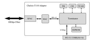
Figure 1. Chelsio T110 Adapter Architecture
