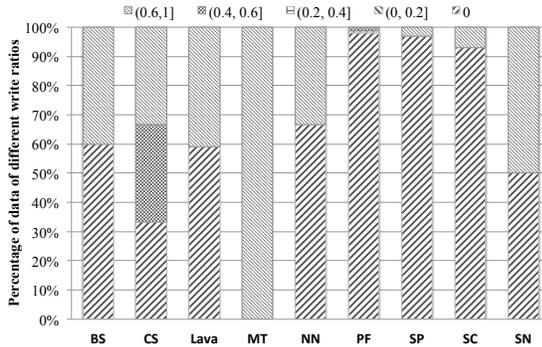
Fig. 5: Write Intensity Distribution of Working Set Data
