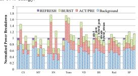
Figure 6: Power comparison among DDR, PCM and STT-RAM
