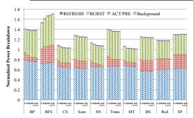
Figure 4: The impact of Row Buffer Locality on Power
