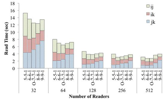
Fig. 8: Dynamic Subchunking Performance; O-7-7-1 (49 subchunks) is our calculated value using the Optimized Chunking formula. We compare the performance with other variation of chunking from 25 (5-5-1) to 81 (9-9-1) subchunks
