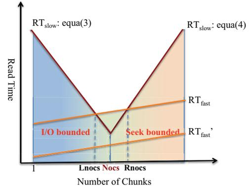
Fig. 2: The Read Time vs. the Number of Chunks
