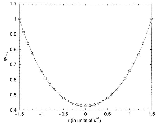
FIG. 3. The electric potential in an electrolyte between two infinite charged parallel flat plates; the solid line is the analytic solution and the circles are the simulation results with  $10^5$  random walks and the absorption layer  $\delta = 10^{-4}$ . Here,  $r$  is the distance from the mid-point of the plates and  $\kappa$  is the inverse Debye length.
