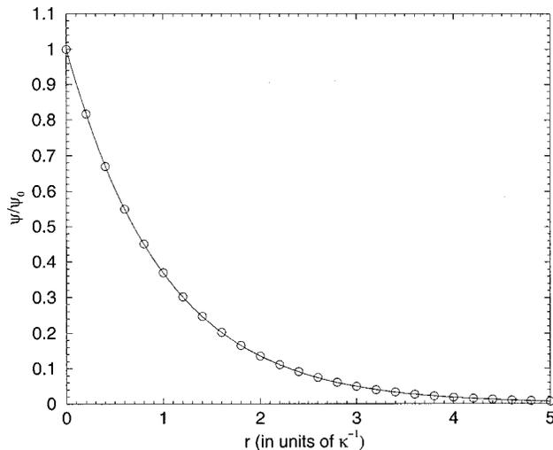
FIG. 2. The electric potential away from an charged infinite flat plate in an electrolyte; the solid line is the analytic solution and the circles are the simulation results with  $10^5$  random walks and the absorption layer  $\delta = 10^{-4}$ . Here,  $r$  is the distance to the plate and  $\kappa$  is the inverse Debye length.
