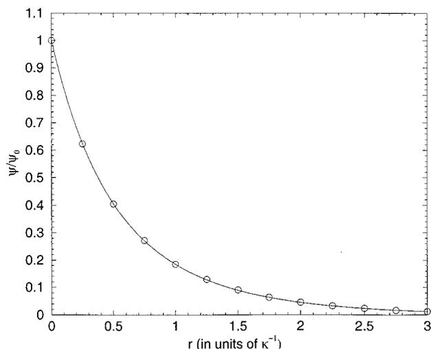
FIG. 5. The electric potential away from the surface of a charged sphere in an electrolyte; the solid line is the analytic solution and the circles are the simulation results with  $10^5$  random walks and the absorption layer  $\delta = 10^{-4}$ . Here,  $r$  is the distance from the surface of the sphere with unit radius and  $\kappa$  is the inverse Debye length.
