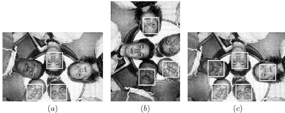
**Fig. 1.** An example of the face detection procedure. (a) The input image with upright detections. (b) The rotated input image with detections using the shuffled spectral histograms. (c) The final detection result by combining that in (a) and (b).
