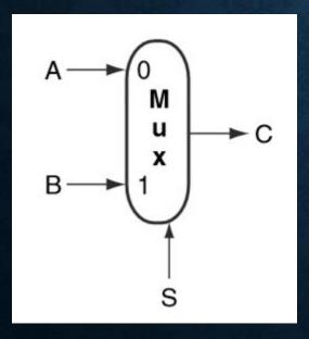
The multiplexor on the left has two input values, A and B. There is an additional input value S, the *selector* (or *control*) value. The selector value determines which of the input values, A or B, will be used as the output value.
