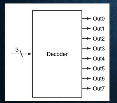
A decoder essentially translates the input signal into a signal that corresponds to the binary value of the *n*-bit input.
