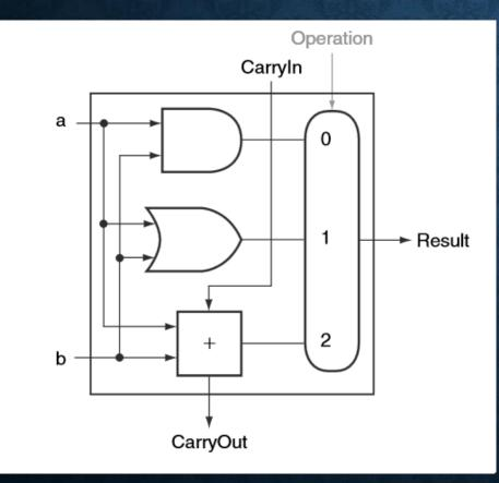
Once we've implemented the CarryOut and Sum logic functions, then we can combine our adder (shown here as a black box again) with the logical operations to create a simple 1-bit ALU.
