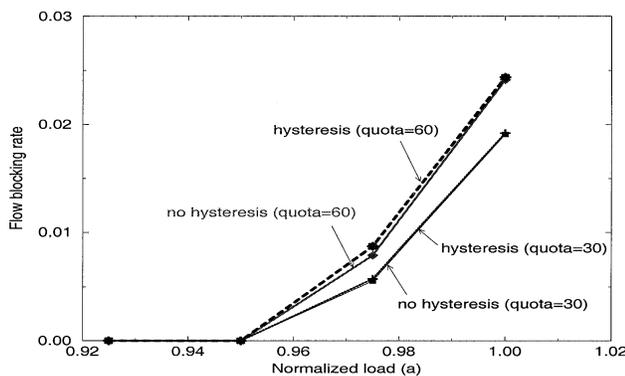
**Fig. 14** Effects of hysteresis on flow blocking rates ( $C = 3600$ ,  $\varepsilon = 0.05$ ).
