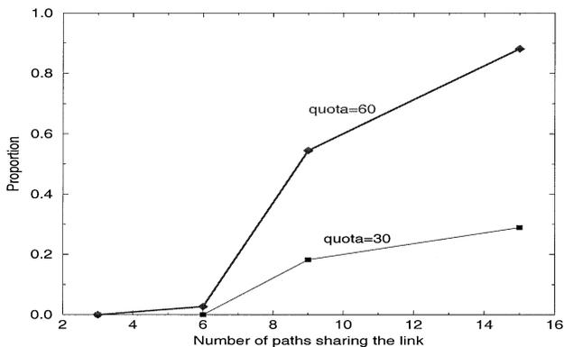
Fig. 10 Proportion of flows accepted in critical mode as the number of paths increases ( $C = 5400$ ,  $a = 0.95$ ).
