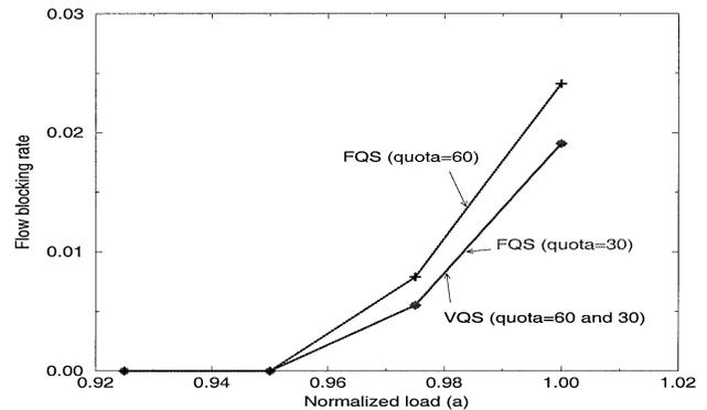
**Fig. 16** Effects of variable quota size on flow blocking rates ( $C = 3600$ ,  $\theta_1 = 0.9$ ).
