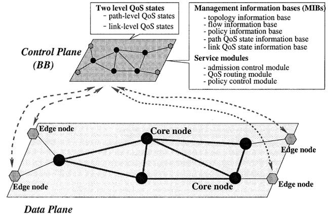
Fig. 1 A bandwidth broker architecture.
