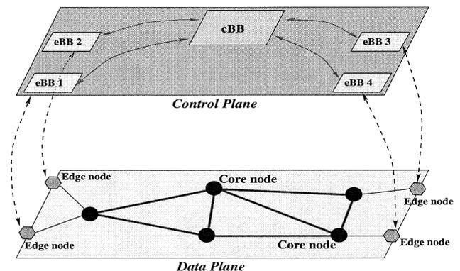
Fig. 11 Multiple bandwidth brokers on the control plane for a network domain.
