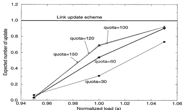
**Fig. 8** Expected number of link-level QoS update per-accepted-flow ( $C = 5400$ ).
