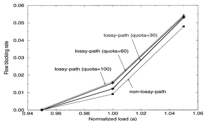
Fig. 12 Flow blocking rate of the non-lossy-path and lossy-path models ( $C = 5400$ ).
