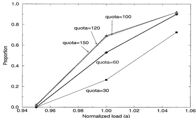
**Fig. 7** Proportion of flows accepted in critical mode ( $C = 5400$ ).
