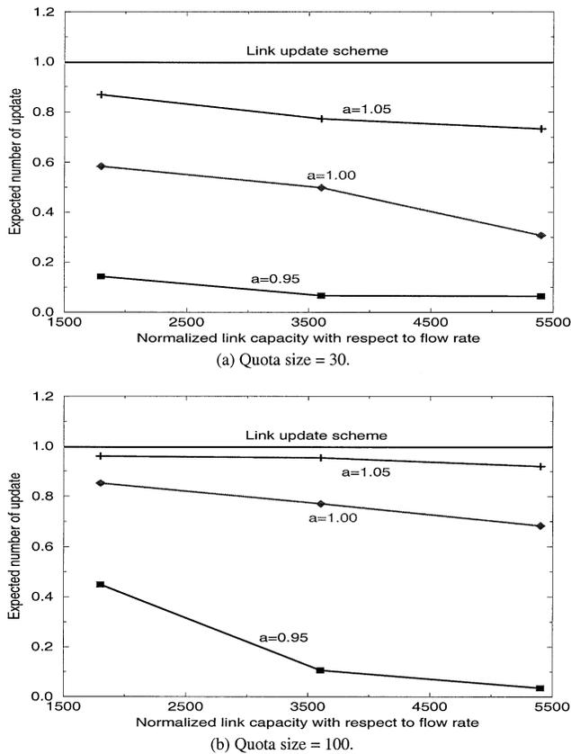
Fig. 9 Expected number of link QoS state updates as the network capacity increases.
