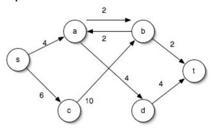
We are given a directed graph (V, E) with a non-negative capacity c for each edge (u, v) in E. The numbers on the *edges* give the capacities, in the above figure. We can take the capacity for edges *not in E* as 0. The vertex **s** above is called the *source*, and the vertex **t** is called the *sink*. We want to maximize the flow from the source to the sink by assigning flow values f to each edge satisfying the following constraints:
