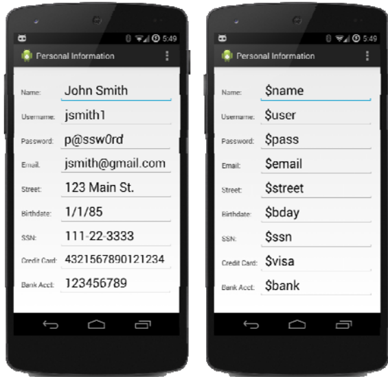
Fig. 2.1. On-screen sensitive data (left) and data protected by masking with cashtag aliases (right).
