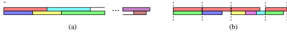
Figure 6. (a). Sending packets in a stream of pairs, which is not practical. (b). Examples of group transmissions, where packets shown at the top are the main packets.
