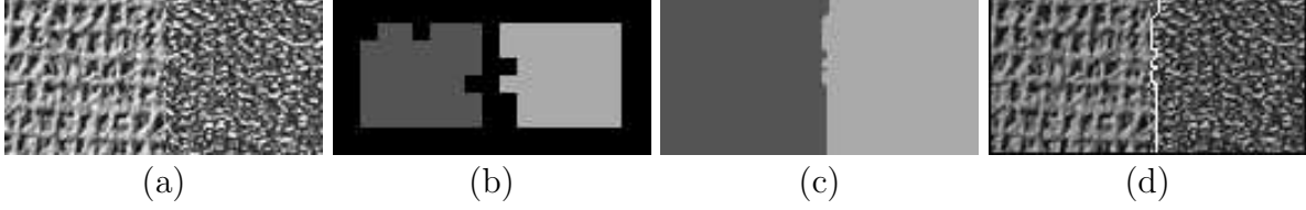
Figure 2.9. Texture image segmentation with representative pixels identified automatically. W^{(s)} is 29 \times 29 , W^{(a)} is 35 \times 35 , \lambda_C = 0.1 , \lambda_A = 0.2 , \lambda_B = 2.0 , \lambda_\Gamma = 0.2 , and T_A = 0.08 . (a) Input texture image. (b) Initial classification result. Here the representative pixels are detected automatically. (c) and (d) Segmentation result and the resulting region boundary.
