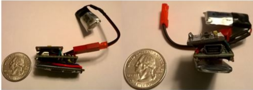
Figure 5.2: Custom build inertial measuring device side and front view
