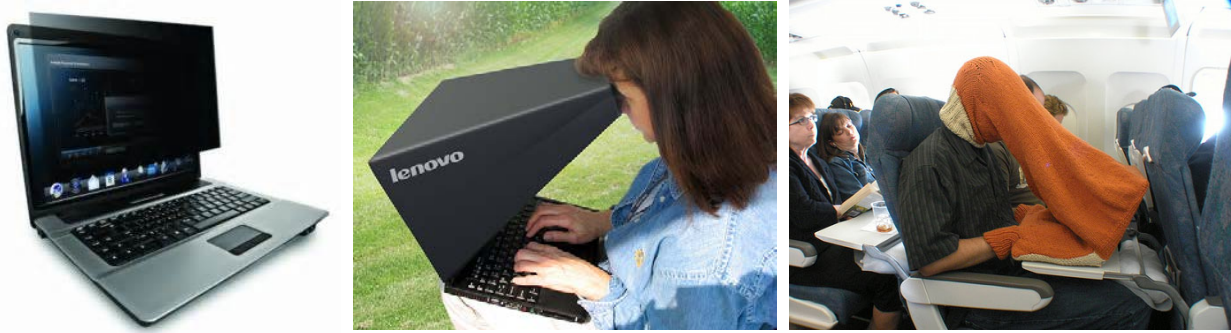
Figure 18: 3M Privacy Filter [67], Lenovo Sun Vision [68], and Compubody Sock [69] screen filters and physical barriers.
