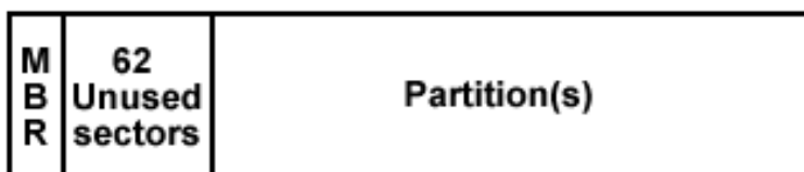
Figure 3.6: Disk layout and master boot record (MBR) space
