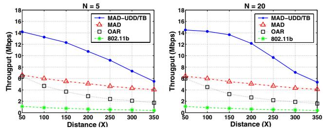
Fig. 7. Network Throughput vs.  $X$  ( $N = 5$  and  $20$ ).
