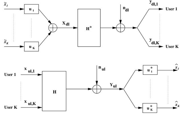
Fig. 1. The downlink and its dual uplink with linear transmitting and receiving strategies.
