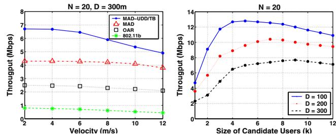
Fig. 8. Network Throughput vs.  $V$ . Fig. 9. Network Throughput vs.  $k$ .
