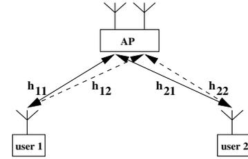
Fig. 2. The AP is equipped with two antennas and each remote user has a single receiving antenna.
