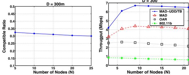
Fig. 6. (a) Compatible ratio vs.  $N$ ; (b) Network throughput vs.  $N$ .
