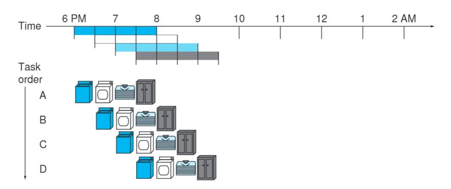
Notice that now we are using parallelism to finish four loads in only 3.5 hours, as opposed to the multi-cycle method which has us doing laundry until 2 AM.
