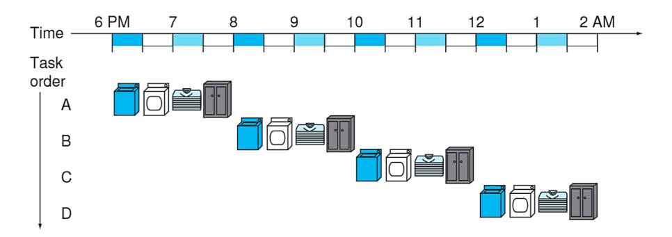
There's no reason why we shouldn't start the next load right after the first load is out of the washer. The washer is available now, after all. This is analogous to pipelining.
