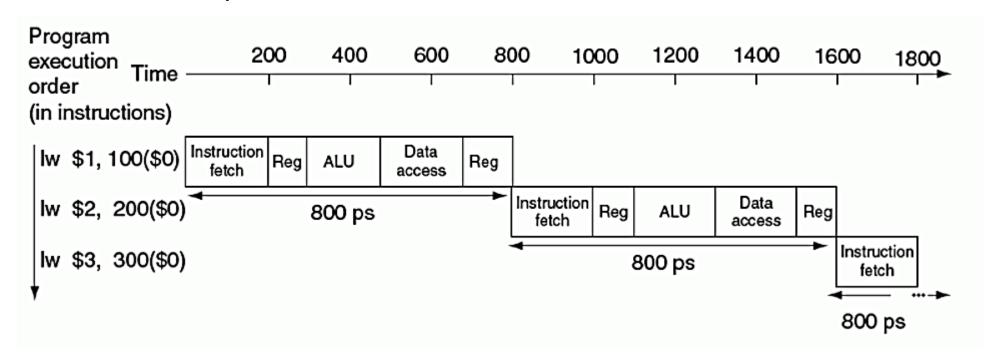
In the pipelining implementation, lw takes 5 cycles totaling 1000 ps. This is because **every cycle needs to be as long as the longest cycle**, which is 200 ps. We start the next instruction as soon as possible. The time between the first and fourth instruction is 600 ps.
