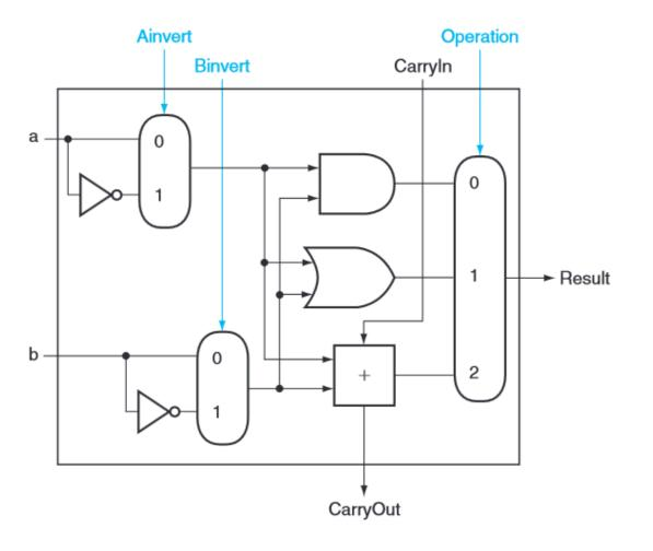
We just need to add support for the SLT (set on less than) operation (and overflow detection).
