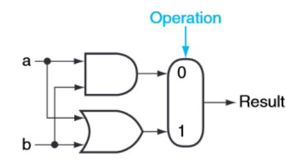
If a has the value 1 and b has the value 0, then a selector value of 1 will cause the result to be 1 while a selector value of 0 will cause the result to be 0.
