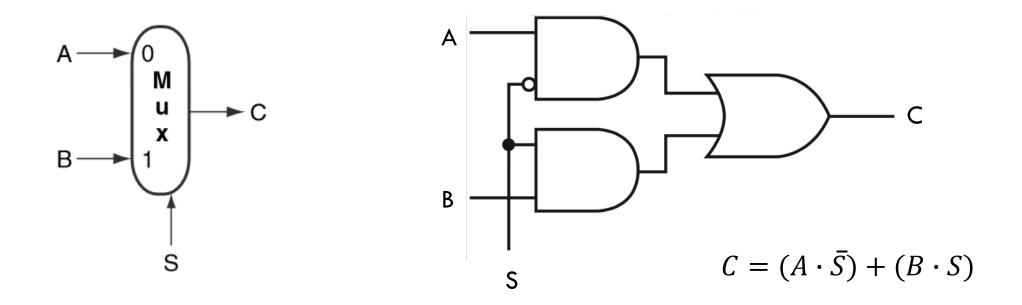
Clearly, with only two data inputs, our selector can uniquely identify the selected input value using only a single selector input. We can select A if S is false (0) and B if S is true (1). But what if we want more than two data inputs?
