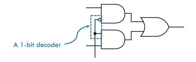
As an example, let's say we want to implement a multiplexor which accepts 4 input bits. We will need 2 selector bits. The selector bits can take on the values 00, 01, 10, 11. Let's say our selector-bits decoder uses the following truth table.
