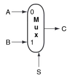
The multiplexor on the left has two input values, A and B. There is an additional input value S, the selector (or control) value. The selector value determines which of the input values, A or B, will be used as the output value.
