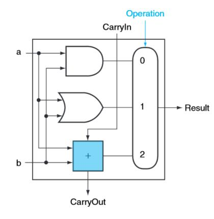
Once we've implemented the CarryOut and Sum logic functions, then we can combine our adder (shown here as a black box again) with the logical operations to create a simple 1-bit ALU.
