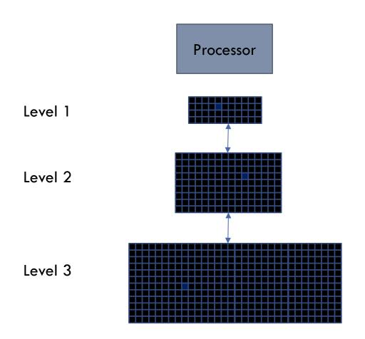
The unit of data that is transferred between two levels is fixed in size and is called a *block*, or a *line*.
