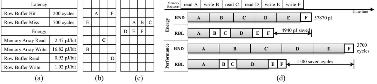
Fig. 5: Conceptual comparison between randomization-based and RBL-aware address mapping schemes. (a) Timing and energy parameters of PCM devices; (b) Data block locations using randomization-based wear leveling; (c) Data block locations using RBL-aware wear leveling; and (d) Performance and energy consumption comparison.
