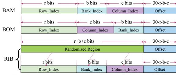
Fig. 2: Address mapping in BAM, BOM and RIB
