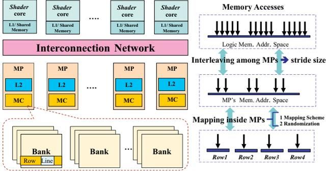
Fig. 1: GPU architecture and hierarchical address mapping
