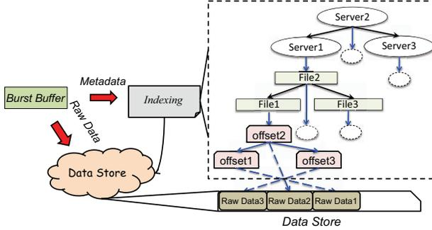
Fig. 5: Server-Oriented Data Organization with Stacked AVL Tree. Segments of each server can be sequentially flushed following in-order traversal of the tree nodes under this server.
