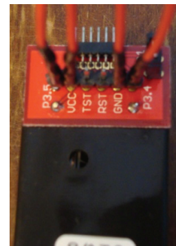
Figure 3: Connect eZ430-RF2480 to Harex LED device using GPIO pins
