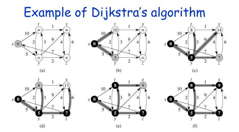
Source is s. Shortest path estimates are in the nodes. The black nodes can be viewed as labeled permanent in that this is the correct shortest path distance to that node. Shaded vertex is next chosen from the priority queue.
