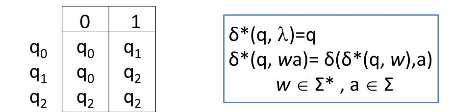
$$\begin{split} \delta^*(q_1, 011) &= \delta(\delta^*(q_1, 01), 1) = \delta(\delta(\delta^*(q_1, 0), 1), 1) \\ &= \delta(\delta(\delta(\delta^*(q_1, \lambda), 0), 1), 1) = \delta(\delta(\delta(q_1, 0), 1), 1) \\ \hline q_0 \\ \delta(\delta(q_0, 1), 1) &= \delta(q_1, 1) = q_2 \end{split}$$
