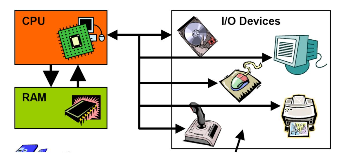
Central processing unit (CPU) → calculate, compute, etc. Random access memory (RAM) → store temporary data I/O device → input/output device
