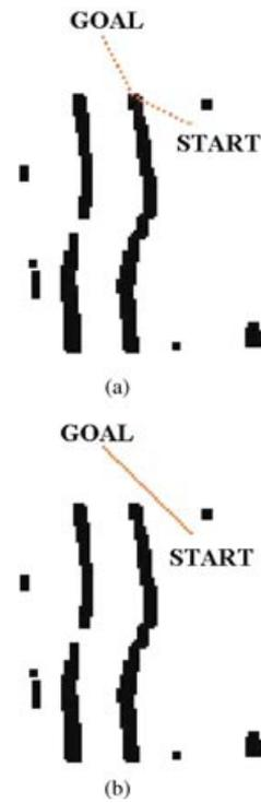
**Figure 14.** (a) Path includes short rut ( $\alpha = 0$ ); and (b) planner avoids the short rut ( $\alpha = 20$ ).
