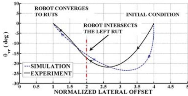
**Figure 30.** Phase portrait from a lateral offset of  $4y_d$  and an orientation of 0 deg.
