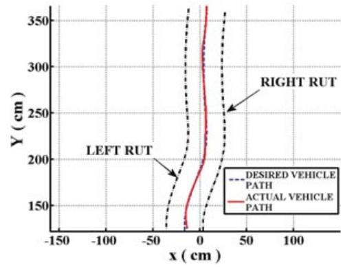
**Figure 33.** Scenario with shallow ruts: desired and actual paths followed by the kinematic center of the robot (cross-track errors: min = 0.001, avg = 0.066, max = 0.262).
