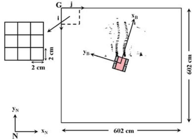
**Figure 11.** Rut grid and coordinate systems.
