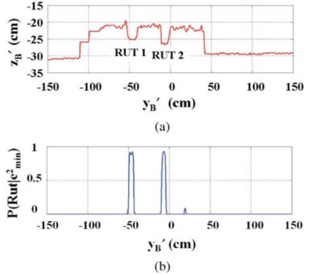
**Figure 10.** (a) Laser data containing two ruts; (b) the corresponding probability estimates of  $P(\text{Rut} | e_{\min}^2)$ .
