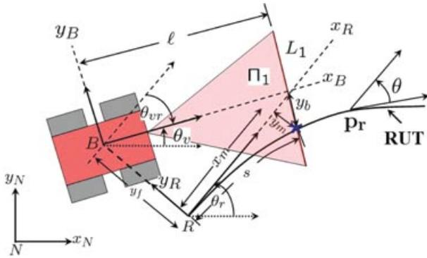
Figure 20. Rut frame coordinates used for rut local modeling.
