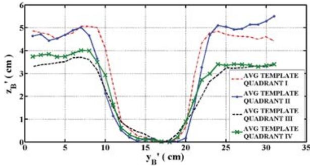
**Figure 9.** Rut templates for the quadrants of the acceptable region for the Pioneer 3-AT.
