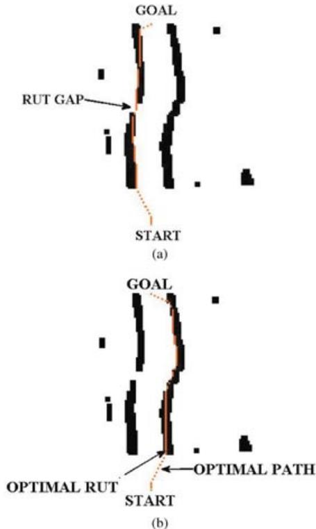
**Figure 13.** (a) Planner selects left rut regardless of gap ( $\alpha = 0$ ); (b) planner selects right rut to avoid gap of left rut ( $\alpha = 20$ ).
