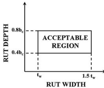
Figure 7. Assumed range of rut widths and depths for traversable ruts (the *acceptable region*).
