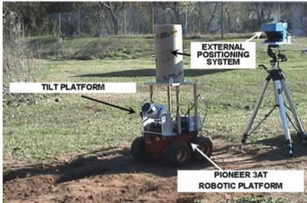
**Figure 24.** Experimental platform: Pioneer 3-AT, tilt platform, and external positioning system.
