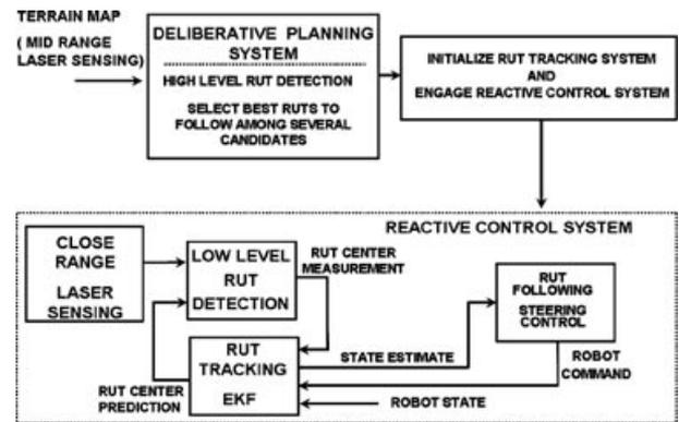
Figure 5. Schematic of the proposed approach to rut detection and following.
