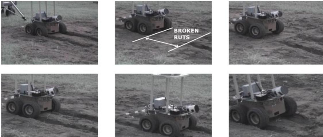
Figure 27. Snapshots of the robot following a broken rut.
