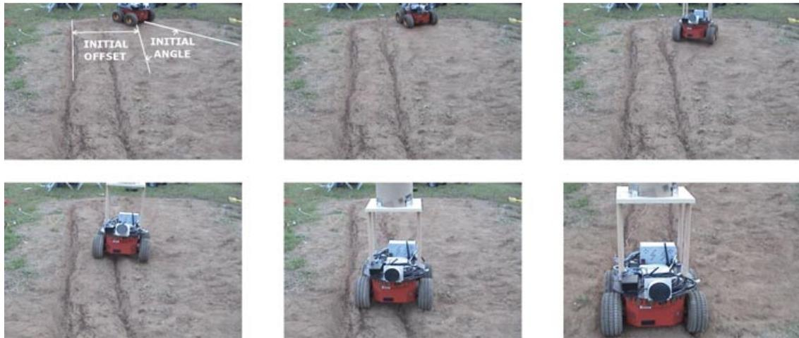
**Figure 31.** Snapshots of the robot approaching the ruts from a lateral offset of  $4.6y_d$  and an orientation of 40 deg.
