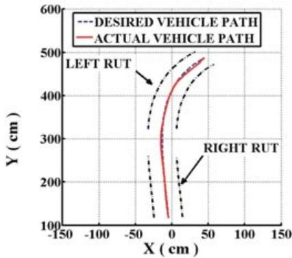
Figure 28. Scenario with broken ruts: desired and actual paths followed by the kinematic center of the robot (cross-track errors: min = 0.002, avg = 0.094, max = 0.495).
