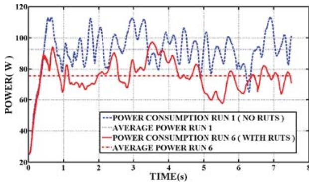
Figure 3. Decrease in power consumption by following ruts (Pioneer 3-AT on sand).
