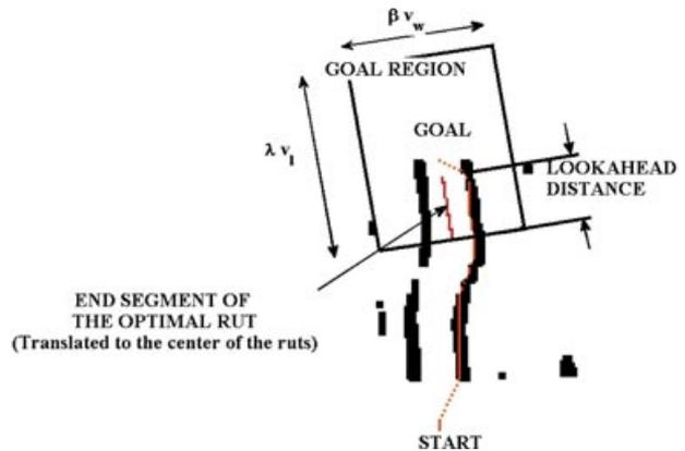
**Figure 17.** Goal region delimiting the area of possible goals that trigger the reactive rut following system.
