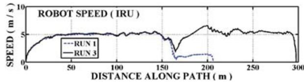
Figure 4. Velocity tracking improvement by following ruts (XUV on mud).
