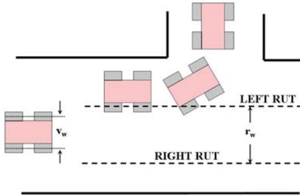
**Figure 18.** A robot using ruts created by a vehicle with a different track width.
