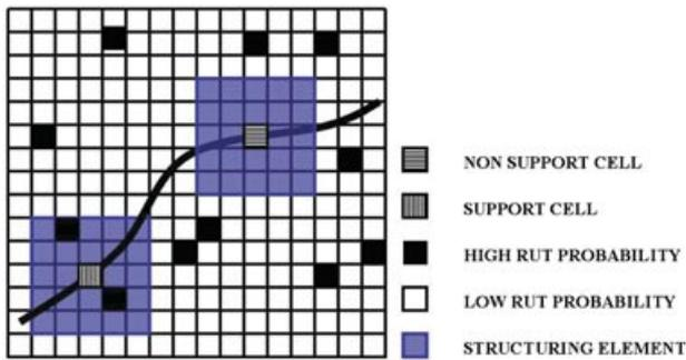
**Figure 15.** Search for support cells along a potential rut using a  $5 \times 5$  structuring element.
