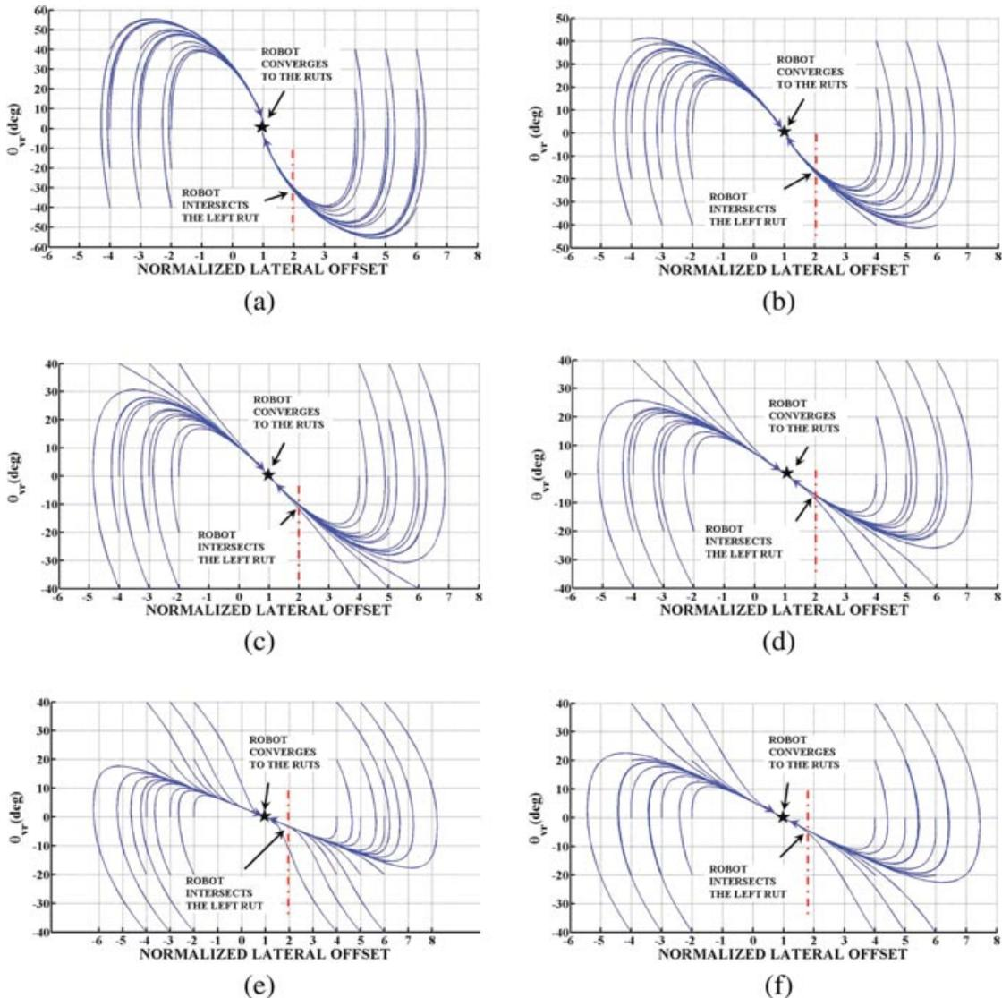
**Figure 23.** Phase portraits for different velocities:  $v_v =$  (a) 0.1 m/s, (b) 0.2 m/s, (c) 0.3 m/s, (d) 0.4 m/s, (e) 0.5 m/s, and (f) 0.77 m/s.
