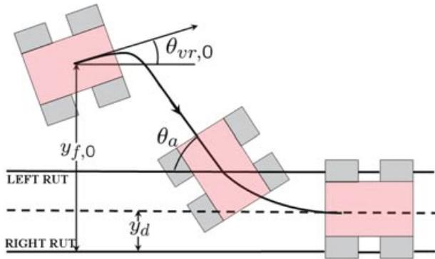
**Figure 22.** Robot converging to a set of ruts from initial nonzero lateral offset and relative orientation, robot-rut.
