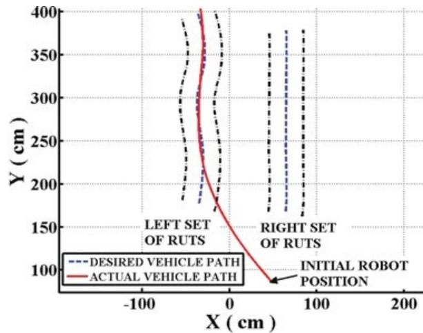
Figure 37. Scenario with multiple ruts: desired and actual paths followed by the kinematic center of the robot (cross-track errors: min = 0.008, avg = 0.162, max = 0.337).
