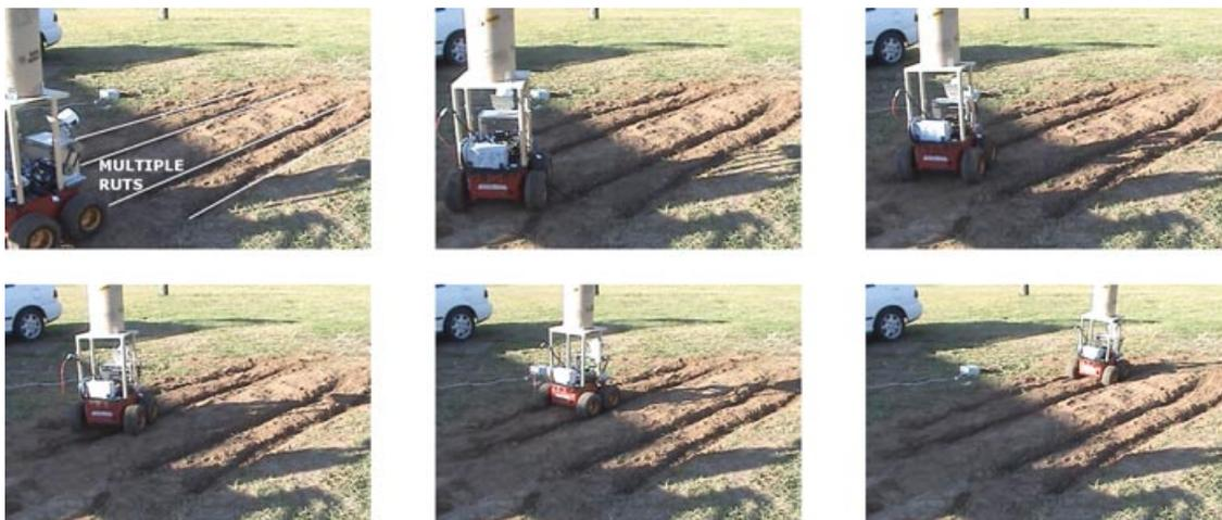
Figure 35. Snapshots of the robot following a chosen set of ruts among different candidates.
