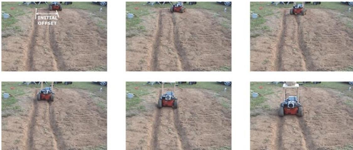
Figure 29. Snapshots of the robot approaching the ruts from a lateral offset of  $4y_d$  and an orientation of 0 deg.
