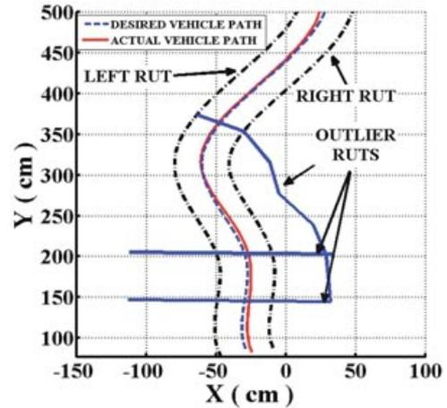
**Figure 26.** Scenario with rut outliers: desired and actual paths followed by the kinematic center of the robot (cross-track errors: min = 0.003, avg = 0.23, max = 0.41).
