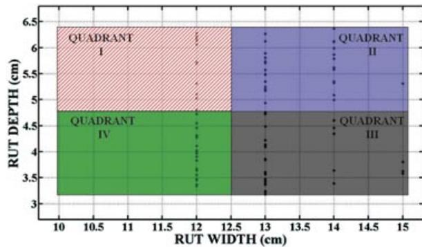
Figure 8. The depth and width of each of the rut samples (indicated by a dot) used to generate the average rut templates for each of the four quadrants of the acceptable region for the Pioneer 3-AT.
