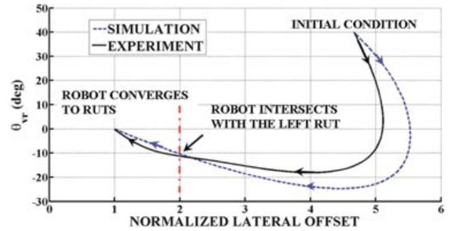
**Figure 32.** Phase portrait from a lateral offset of  $4.6y_d$  and an orientation of 40 deg.
