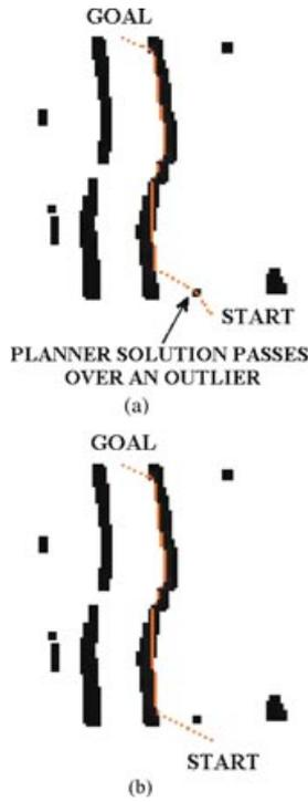
**Figure 12.** (a) Path includes outlier ( $\alpha = 0$ ); (b) path avoids outlier ( $\alpha = 20$ ).
