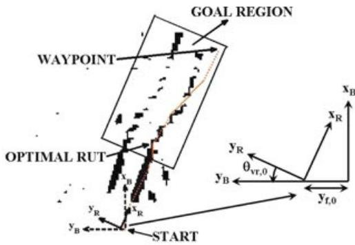
Figure 34. Rut grid used by deliberative system to estimate  $\theta_{vr,0}$  and  $y_{f,0}$ .
