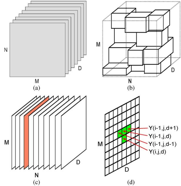
Fig. 1. Illustration of Sun's algorithm. (a) Image volume, composed of an input image with varying disparities. (b) Three-dimensional volume of coefficients with subregioning. (c) Vertical sections. (d) Calculating intermediate volume.
