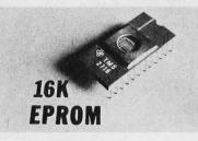
If your 2708 erasable programmable read only memories (EROMS) are filling up fast, here's one answer to the problem: Texas Instruments' 2716, a direct plug-in replacement for the 2708. Each chip contains 16,384 bits of memory and features low power consumption (375 milliwatts typical) and DC noise immunity in both high and low states so that all inputs can be driven by TTL logic without the use of pullup resistors.
