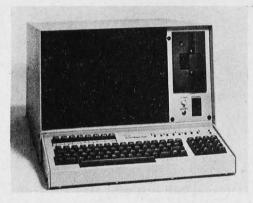
TEI Inc of Houston TX has announced a new processor terminal. Designated the Model MCS-PT, the unit is a self-contained computer system with display and disk storage, keyboard, and a 12 slot motherboard. It may be used either as a stand alone processor or as a processor terminal in a larger system.
