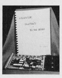
The Center for the Study of the Future has announced an electronic Selectric interface kit designed to work with most Selectric terminals and typewriters using the Tycom adapter. It includes 14 solenoid drivers rated for 24 V (solenoids and power supply are not included in the kit). The price of the kit plus manual is \$325, available from the Center for the Study of the Future, 4110 NE Alameda, Portland OR 97212, (503) 282-5835.
