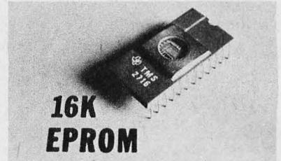
If your 2708 erasable programmable read only memories (EROMS) are filling up fast, here's one answer to the problem: Texas Instruments' 2716, a direct plug-in replacement for the 2708. Each chip contains 16,384 bits of memory and features low power consumption (375 milliwatts typical) and DC noise immunity in both high and low states so that all inputs can be driven by TTL logic without the use of pullup resistors.
