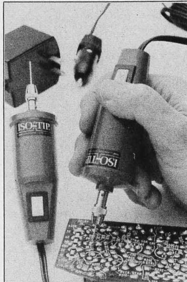
Here is a device that should prove useful for the fabrication of printed circuit boards, as well as other applications involving the drilling and cleaning of small holes. The Wahl ISO-TIP electric drill is less than 5 inches (12.7 cm) long with drill bit removed and is designed to fit into tight corners. The on-off switch provides both intermittent and locked modes of operation, and the power cord is 10 feet (3.04 meters) long.
