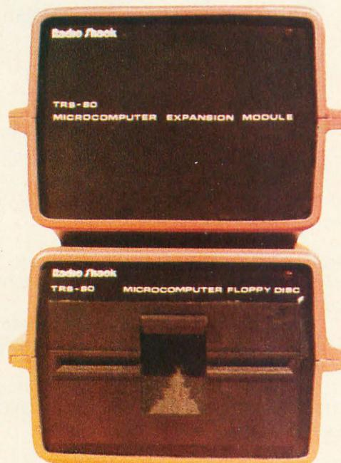
Photo 4: A closeup of the forthcoming microcomputer expansion module and disk drive.
