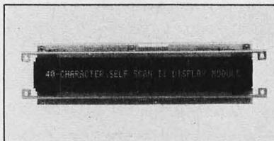
The Electronic Components Division of Burroughs Corporation, POB 1226, Plainfield NJ 07061, has introduced this new single line 40 character version of Self-Scan II technology, intended for use in any product where a limited size alphanumeric display is required. Special effects include left or right data entry, moving message effects, blinking subfields within the 40 character line, etc. Self-Scan is a registered trademark of Burroughs Corporation. ■
