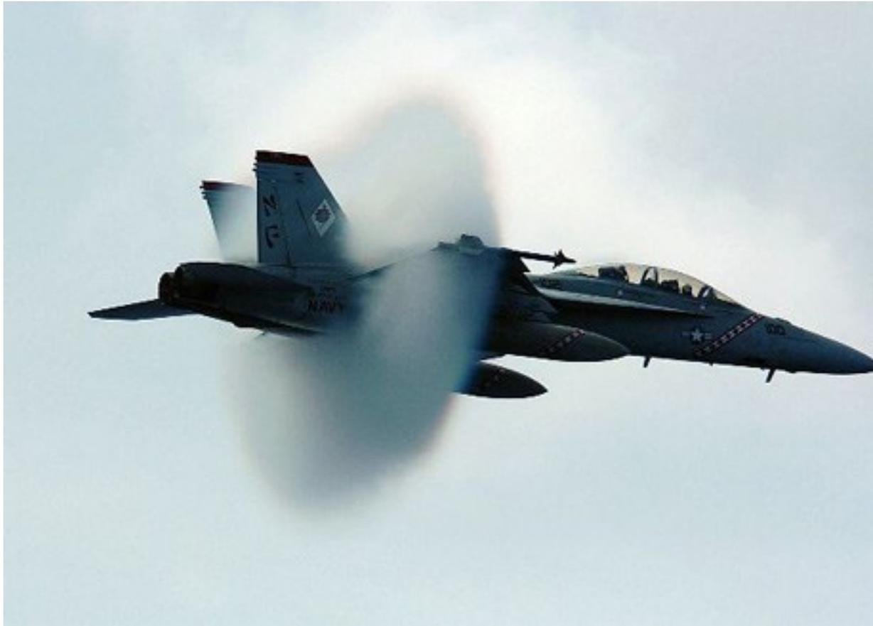
F/A-18F Super Hornet breaking the sound barrier
