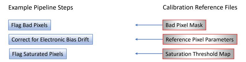
Reference files often change as a result of instrument/detector aging, as well as better understanding and analysis of calibration data.
