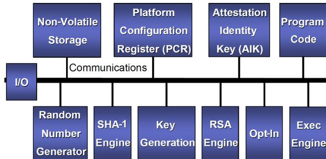
Fig. 2. The components of a Trusted Platform Module.
