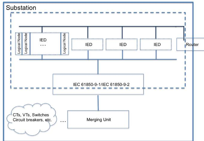
**Fig. 1.** An illustration of a substation in which the communication between IEDs is IEC/TR 61850-90-5 compliant.
