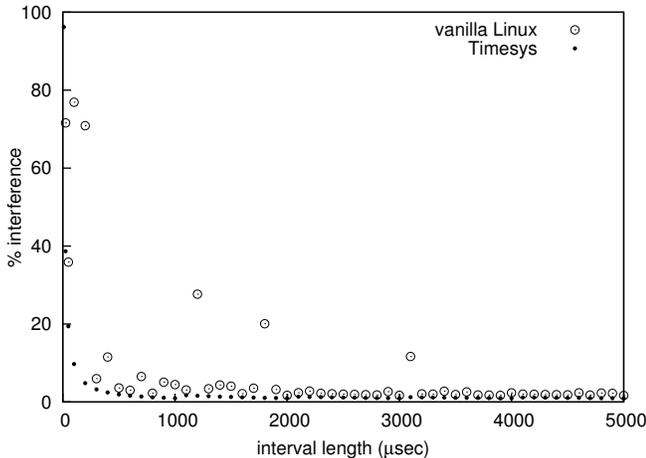
**Figure 4.** Observed interference with no network traffic.
