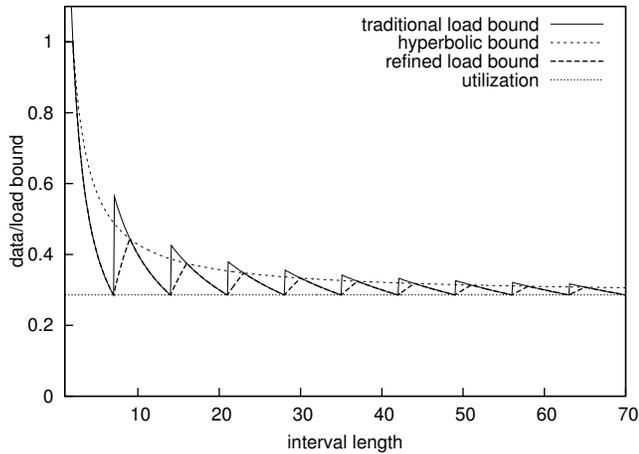
**Figure 2.** Load bounds for a periodic task with  $p_i = 7$  and  $e_i = d_i = 2$ .
