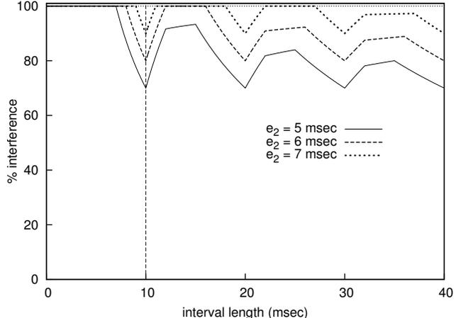
**Figure 9.** Sum of load-bound functions for  $\tau_1$  and  $\tau_2$ , for three different values of the execution time  $e_2$ .
