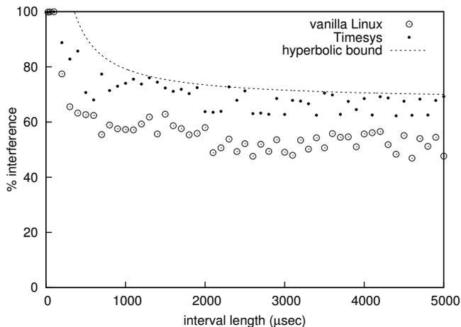
**Figure 5.** Observed interference with ping flooding, including reply.
