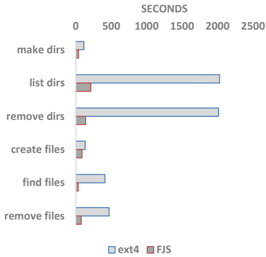
Figure 5.2.5: Comparison of SMR HDD performance between FJS and ext4 running Filebench microbenchmarks.
