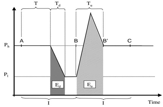
**Figure 2:**  $T \leq I < T + T_u$ . Accesses arrive at times A, B, and C. Accesses are actually performed at times A, B', and C.
