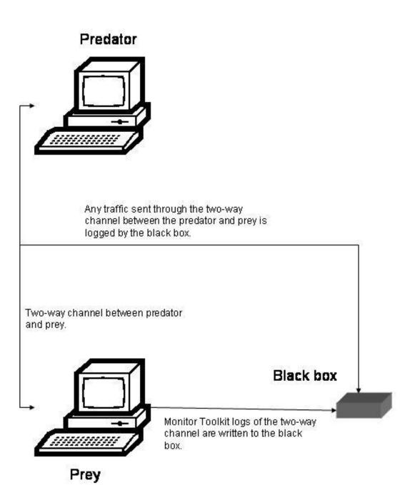
Figure 4.1 PAPA System black box: Illustration of Monitor Toolkit logging. The bidirectional arrows depict data flow in both directions. The unidirectional arrow between the Prey and the black box illustrates that data can only be written into write-protected logs.
