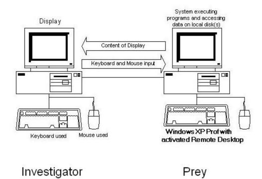
Figure 8.1 Transfer of data using Windows Remote Desktop: The Investigator's computer sends keyboard and mouse input data to the Prey's computer which is executed on the Prey's computer. Data that would normally be displayed on the Prey's monitor is instead sent to the Investigator's machine.
