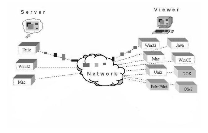
Figure 8.2 VNC server interacting with a VNC client: An illustration showing how VNC software can be used across platforms to view and interact with a computer running a VNC Server using the VNC Viewer on another machine.
