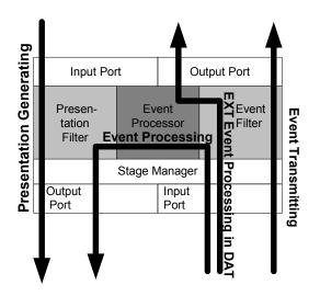
Figure 4.5 Possible dataflows in a stage
