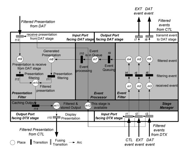
Figure 4.9 *PT<sub>CTL</sub>* : CTL stage with PT-net
