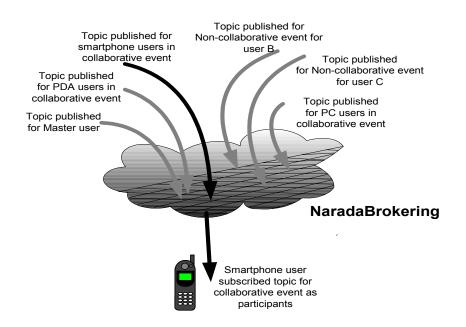
Figure 7.7 Filtering collaborative message for smartphone user in the NaradaBrokering
