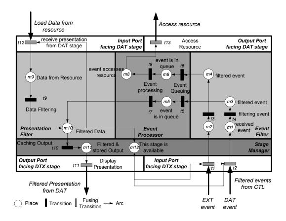
Figure 4.10 *PT<sub>DAT</sub>* : DAT stage with PT-net
