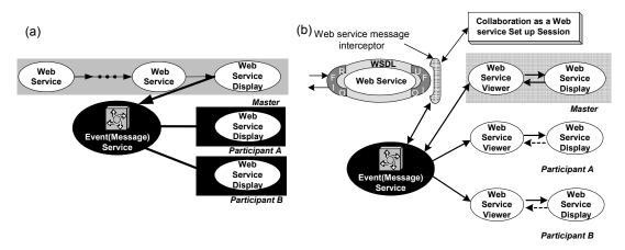
Figure 7.1 Deploying Collaboration model as Web Service (a) Shared Display model as Web Service (b) Shared Output model as Web Service
