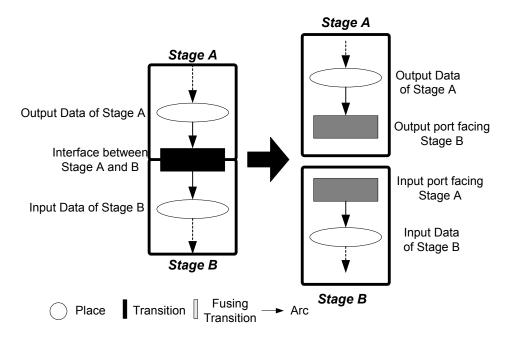
**Figure 4.4 Defining Interface with Fusing Transitions**
