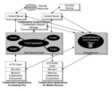
Figure 7.3 Architecture of the Carousel Web service
