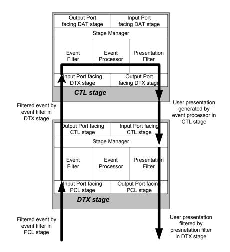
Figure 3.7 Architecture of a Stage in MDPA with dataflow of CTL event
