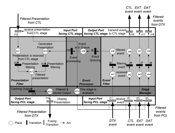
Figure 4.8 *PT<sub>DTX</sub>* : DTX stage with PT-net
