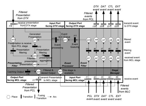
Figure 4.7 *PT<sub>PCL</sub>* : PCL stage with PT-net
