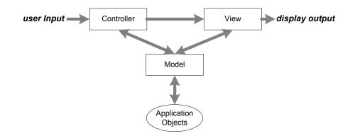
Figure 2.2 The MVC architecture
