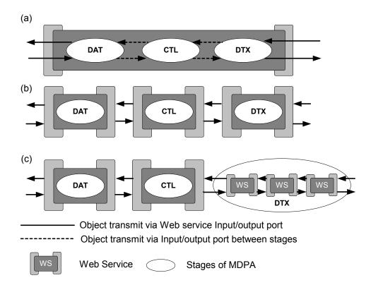
Figure 3.10 Various Styles of Packaging Stages with Web service infrastructure
