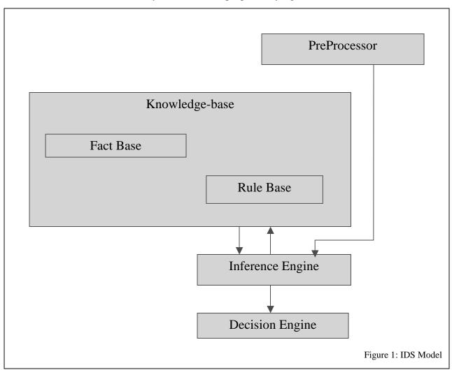
Basic Intrusion Detection System Model as proposed by Ilgun, Kemmerer [95]:
