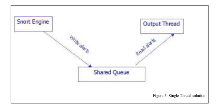
For n Threads, the number of threads is determined by the Snort user (typically a network administrator) with the command line argument of Snort. Snort Engine is not concerned with the number of threads. It will just write the output to the shared queue and carry on. The Output Threads take turns taking care of the alert messages.
