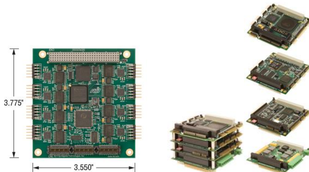
Figure 4 - A basic PC/104 stack http://www.rtd.com/PC104
