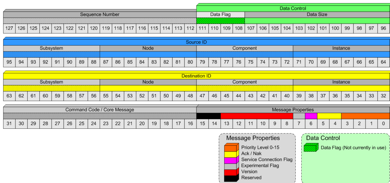
Figure 59 - Joint Architecture for Unmanned Systems (JAUS) Header that accompanies all JAUS messages
