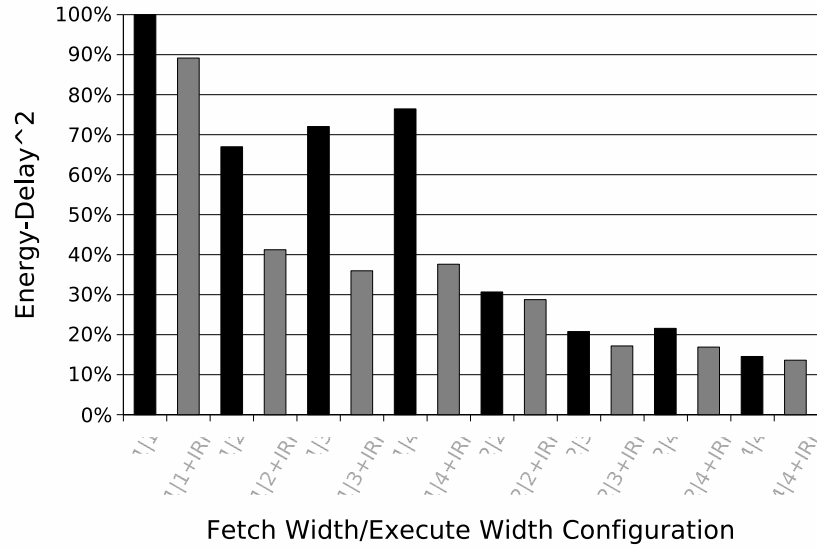
Figure 2.41: Energy-Delay 2 for Asymmetric Pipeline Bandwidth
