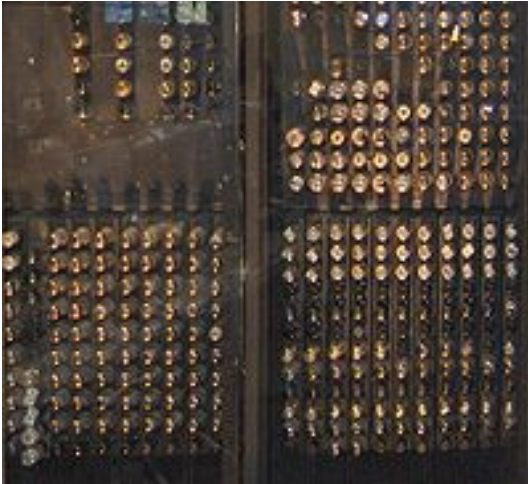
Figure: Tubes from the ENIAC
