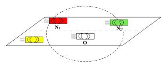
Figure 2 Groupwise communication in the TSVC scheme
